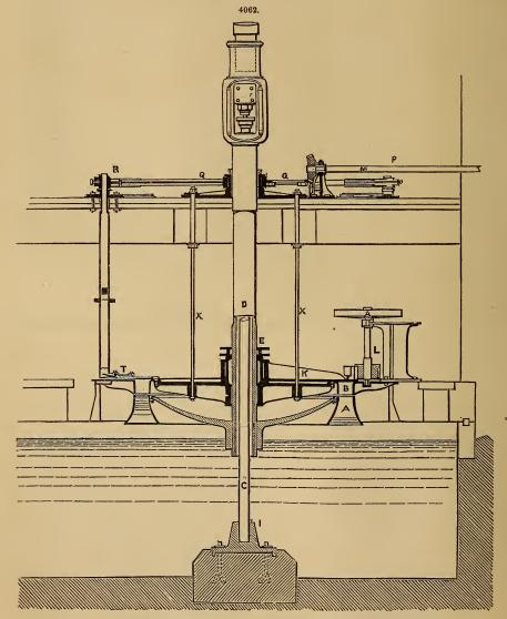
with two independent register-valves. But in many cases M. Girard prefers to supply the wheel upon only  $\frac{1}{4}$  or  $\frac{1}{5}$  of its circumference in order that its orifices may be larger, and so, less liable to
